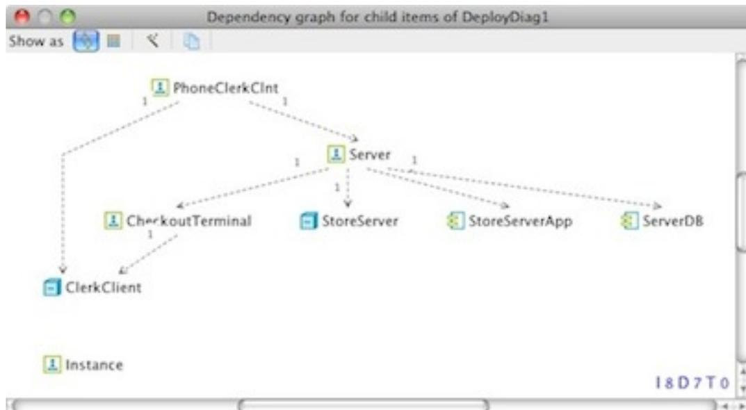
The contained components within nodes use the dependency-type 'deployed-in' and NOT node containment.
