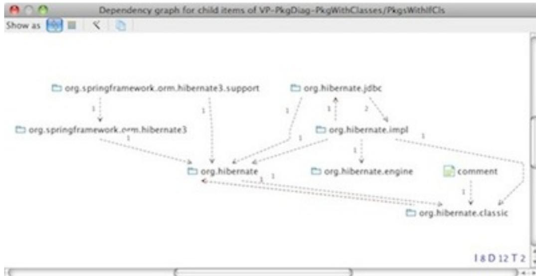
In the above dependency graph, not all level of nodes are shown, only one level is shown. This problem will be fixed in the core ReStructure101g product. But the architecture diagram included below, shows all the levels of the nested nodes, which includes interface classes of some of the packages.
